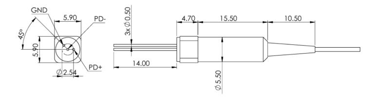
Standard Package for Infrared Band. For other wavelength band, size may vary due to special detector configurations.
